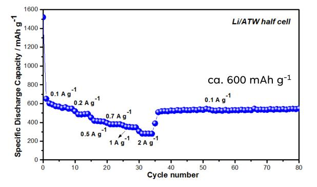
When the current density rolls back to 0.1 A g<sup>-1</sup>, the electrodes show the excellent capacity retention of 100%.
